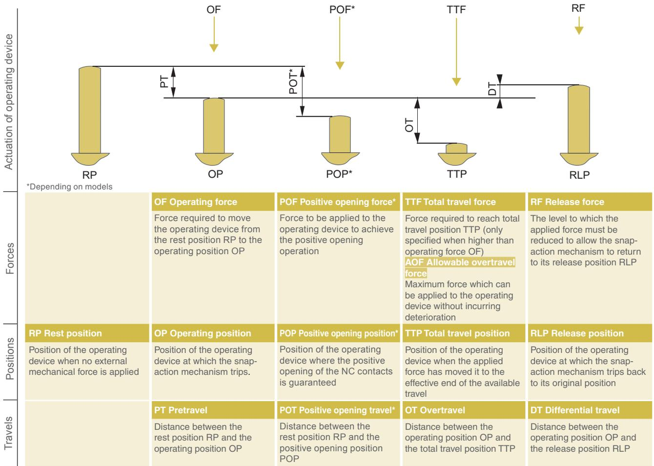
The reference point for the figures given for travels and forces is a point F located on the top of the plunger in the case of a plain microswitch, or, generally, 3 mm in from the end of a flat lever. The reference point for the positions is one of the fixing holes, unless otherwise indicated.
