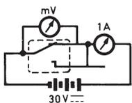
This is the electrical resistance measured at the terminals of the switch when the contacts are closed. It consists of the (variable) resistance of the contact point and the (fixed) resistance of the current carrying parts.
