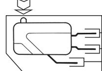
Unless otherwise indicated, they are intended for Class I devices and their envelopes provide basic insulation. Microswitches for Class I equipment are also suitable for Class II equipment, with appropriate installation conditions in the equipment.
