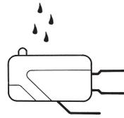
Degrees of protection provided by enclosures against access to hazardous parts, against ingress of solid foreign objects and against harmful ingress of water are defined in IEC 60529 by an IP code followed by two digits.
