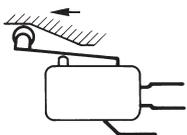
When the roller lever is laterally approached, force should preferably be applied in the direction shown.
