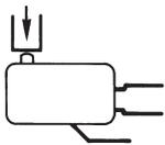
The plunger should preferably be actuated along its axis (front actuation). However, the majority of our microswitches can accept lateral approach provided the angle of actuation is not more than 45°.
