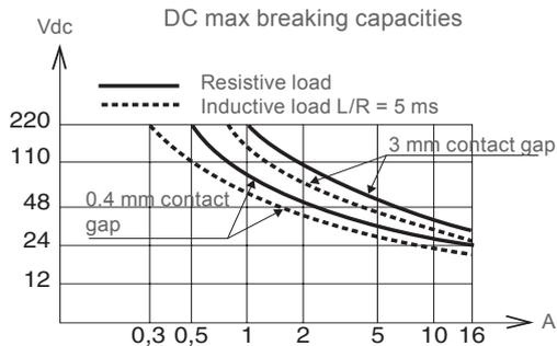
DC breaking capacity can be significantly increased by using different means, if necessary in combination:
