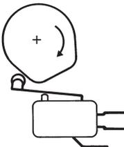
Where the movements involved are fast, the ramp should be designed to ensure that the operating device is not subjected to any violent impact or abrupt release.
